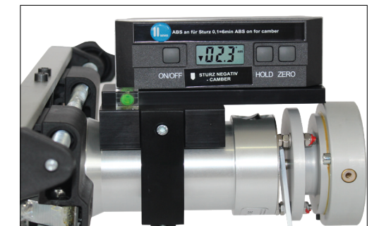
Electronic measure of camber and castor
